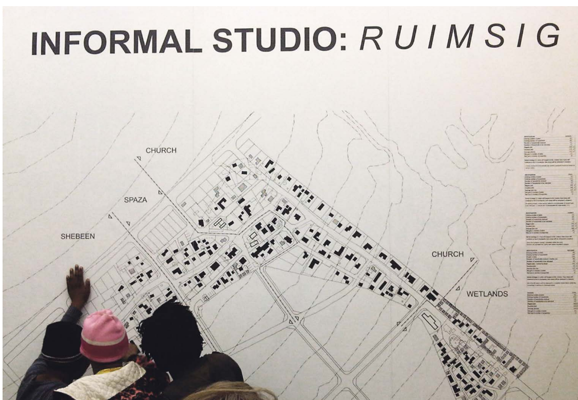
Re-blocking map for Ruimsig showing remaining structures (in solid black) and re-located structures (grey) © 26'10 south Architects
